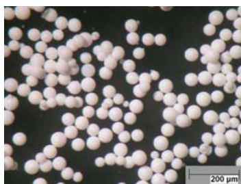
Figure 1: Optical micrography of the unmodified S-DVB copolymer (magnification: x50)
